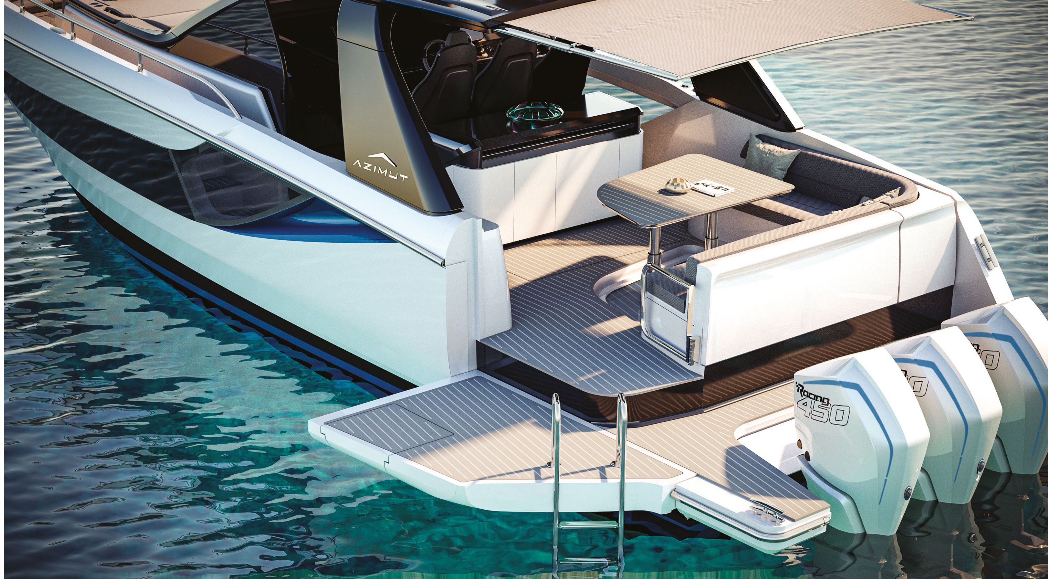
Portside aft bulwark folds out to enlarge the space offering an easy access to the sea.
