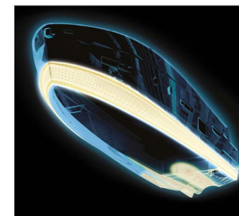
Dual Mode semi-planing hull with tunnel, skeg and vertical bow (Magellano Collection)
